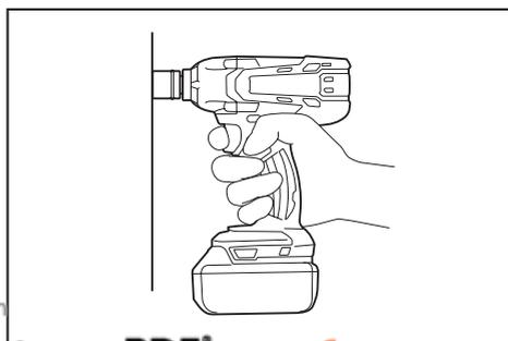
Put the tool firmly on the surface and place the impact socket over the bolt or nut. Turn the tool on and fasten for the proper fastening time.
