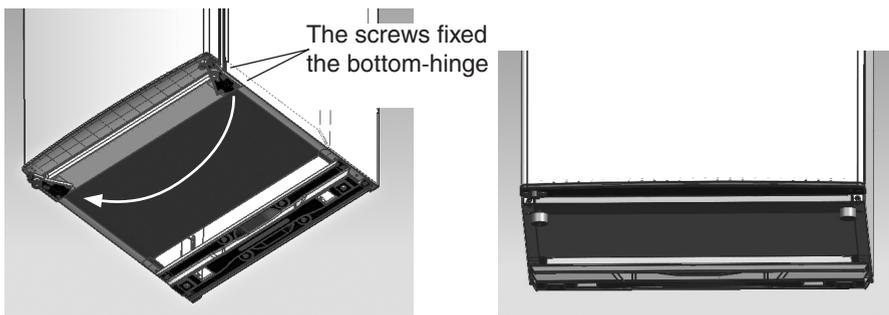
7. Set the door right position, fix the top-hinge and then the roof cover.
