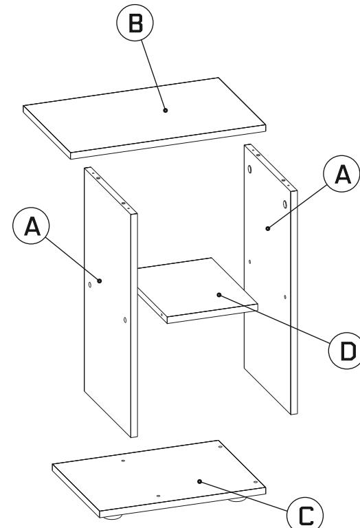
**A** 542 x 296 x 16 [x2]**B** 300 x 470 x 16 [x1]**C** 300 x 400 x 16 [x1]**D** 294 x 218 x 16 [x1]
